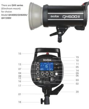
(1)AC Power Socket (2)Sync Cord Jack (3)Power Switch (4)Modeling Lamp Output Controller (5)Flash Output Controller (6)Modeling Lamp Button (7)GR/CH Button (8)Slave Model Button (9)Test Button (10)Digital Display (11)Modeling Lamp Indicator (12)Buzz Button (13) Custom Function Button (14)Test Indicator Lamp (15)Light Sensor (16) Wireless Control Port (17)Fuse (18)Mounting Bracket (19)Umbrellas Input (20)Direction Adjusting Handle
